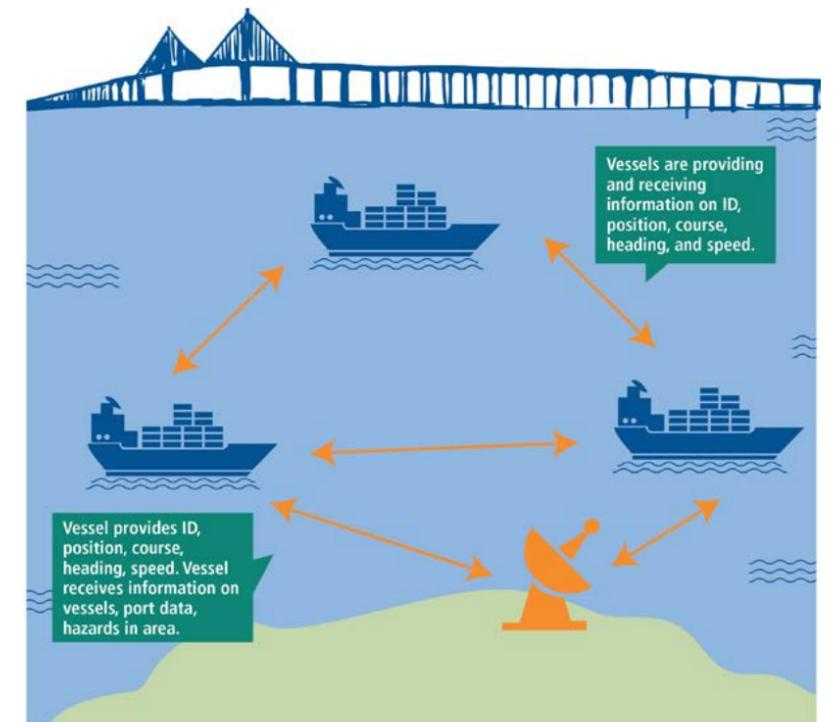
How AIS Works: An Automatic Identification System (AIS) deploys small transponders on ships to continuously relay signals about their position to other vessels, shore stations or satellites equipped with AIS receivers. The information is displayed on an electronic chart. AIS technology is universally used in the global maritime industry to prevent ship collisions. Recreational mariners, especially those who cruise long distances, also are adopting its use.
